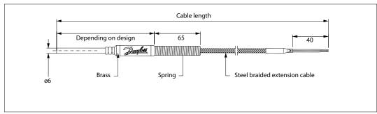
Pocket for MBT 5111 – ø6 version ((To be used together with compression fitting)
